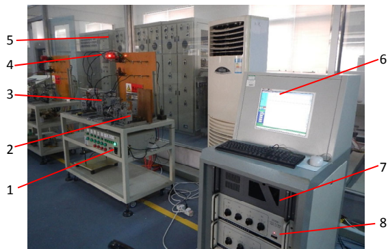
1: control cabinet; 2: operating mechanism; 3: circuit breaker undergoing testing with angular displacement sensor and optical fiber thermistor temperature sensors; 4: alarm lamp; 5: impedance cabinet used for loading; 6: user interface; 7: signal processor; 8: range transform amplifier
