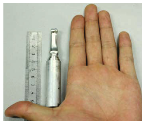
Fig. 15 Finished artificial finger bone part
