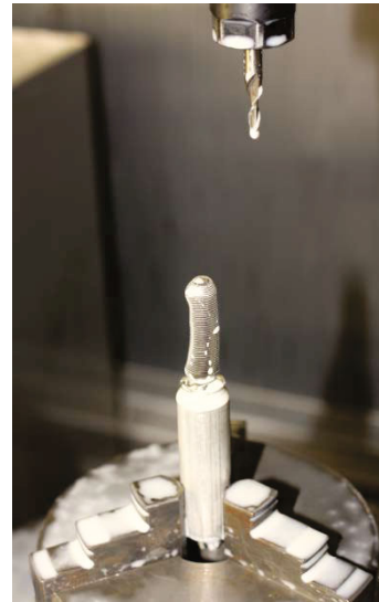
Fig. 13 Artificial finger bone model being machined
