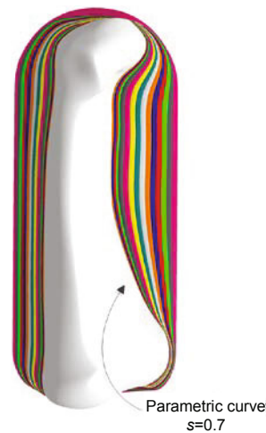
Fig. 10 Profile view of all levels Points are sampled from the parametric curve s=0.7 for cutting depth analysis
