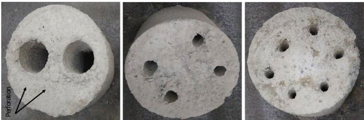
Fig. 10 Concrete blocks, with different numbers and sizes of holes, used in packed bed solutions for TES [108]
