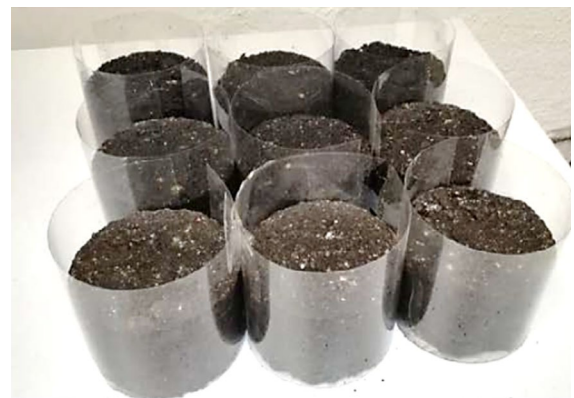
Fig. 2 Curing of cylindrical specimens
