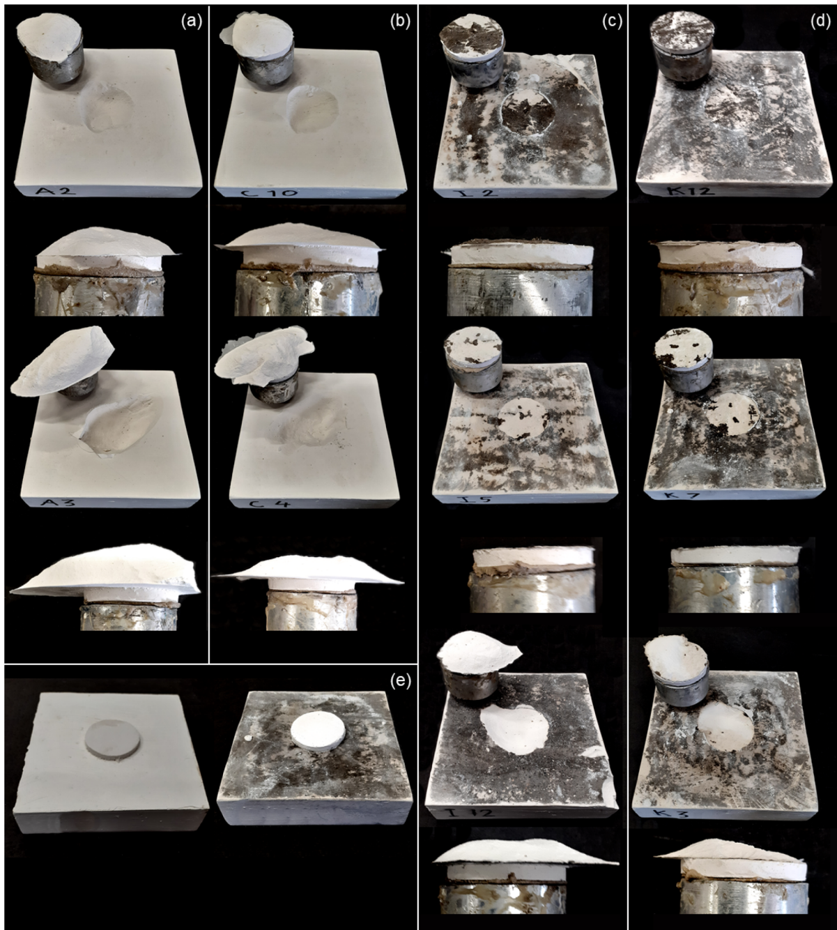
Fig. 9 Tested specimens from groups AP-CB, AP-QF-CB, AP-DB, and AP-QF-DB. a Group AP-CB, cohesive failure of base material. b Group AP-QF-CB, cohesive failure in bases. c Group AP-DB, partial cohesive failure of base material (top, middle) and cohesive failure (bottom images). d Group AP-QF-DB,
