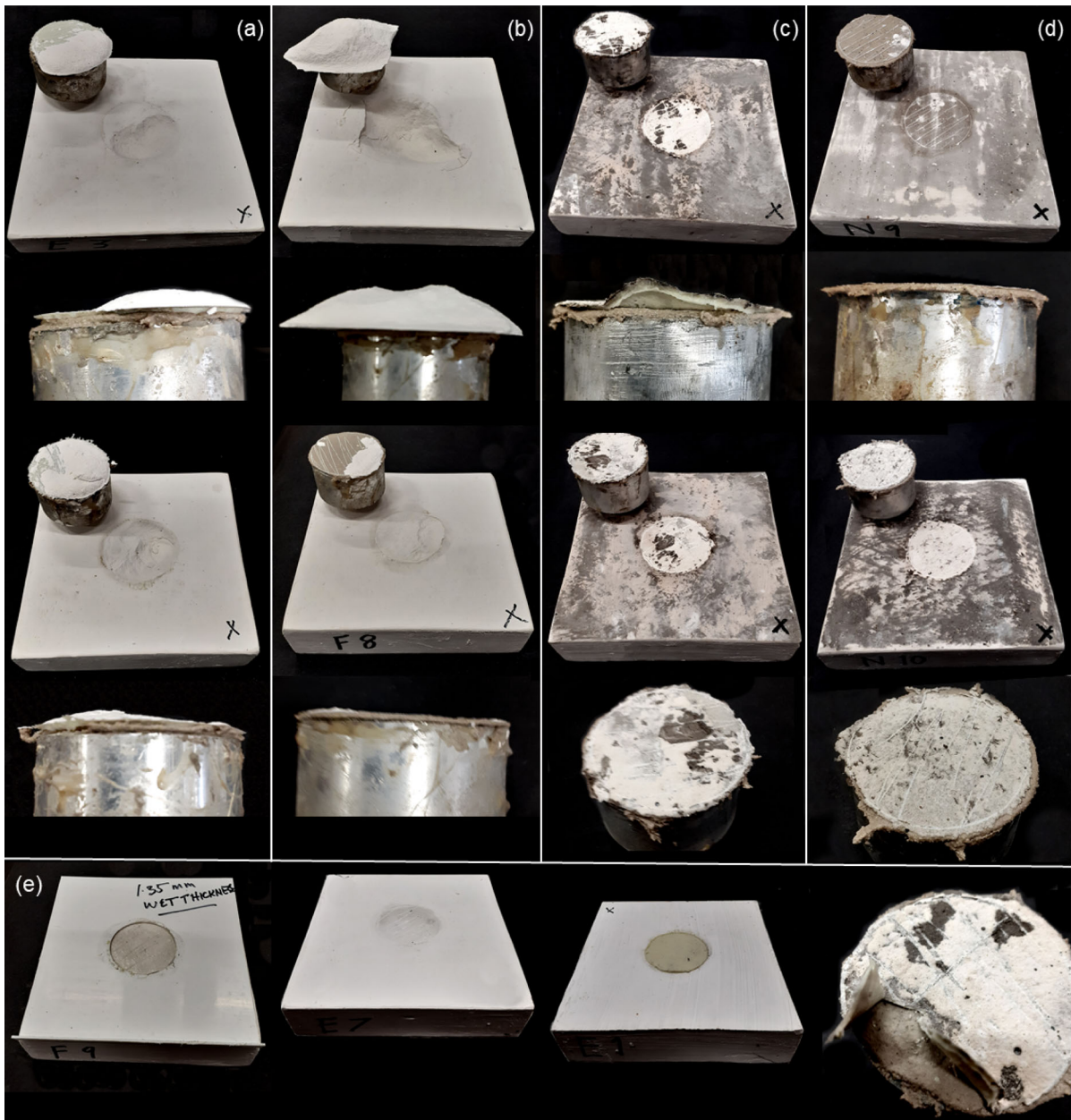
Fig. 10 Tested specimens from groups AG-KF-CB, AG-P-CB, AG-KF-DB, and AG-P-DB. a Group AG-KF-CB, adhesive and cohesive failure with partial cohesive failure of base material. b Group AG-P-CB, cohesive failure with base material removed (top) and partial cohesive failure of base material (lower). c Group AG-KF-DB, partial cohesive failure of base
