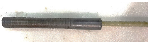
Fig. 5 Grooved steel pipe used for testing GFRP bars
