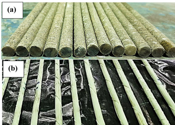
Fig. 1 GFRP bars: a sand coated, b Ribbed
