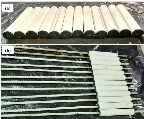
Fig. 4 Actual anchored bars: a prepared pipes, and b GFRP bars placed inside the pipes
