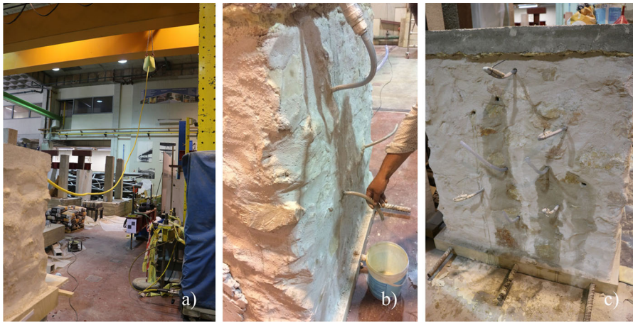
Fig. 2 Injection of specimen: a bucket and hose with mortar during injection, placed at 5 m height, b I 2 (pouring mortar from one of the lower tubes), and c I 1 (with several injection holes)
