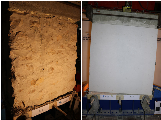
Fig. 9 Rigid body behaviour of a wall strengthened with injection and G-FRCM system (IG 2), both sides view
