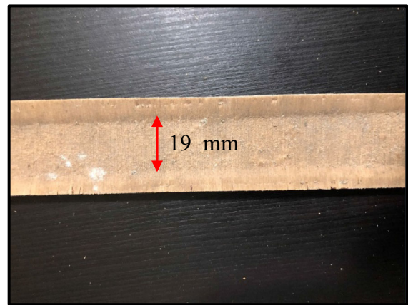
Fig. 6 Impression on ply caused by the application of compressive loads
