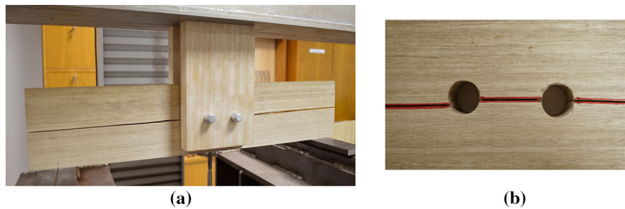
Fig. 4 a Representative failure behaviour of the double-dowel test series; b detail of local failure around the dowels
