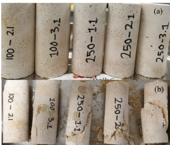
Fig. 6 Triaxial test specimen a before testing (top row), b after testing (bottom row)
