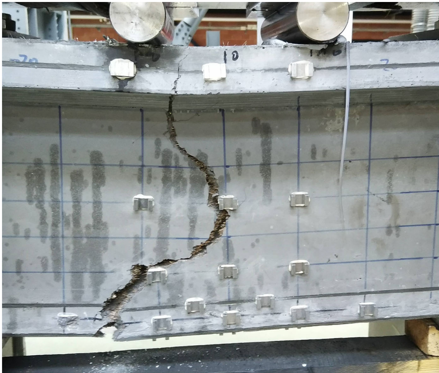
Fig. 5 Mid-span of the beam after failure with critical crack; visible metallic bases of extensometers and gray horizontal line where the DFOs is glued
