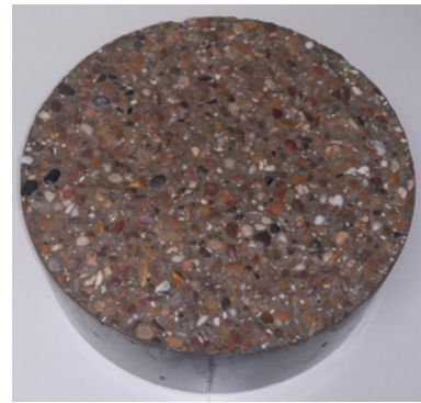
Fig. 4 Abraded test specimen of mixture FC1.5 at 72 h
