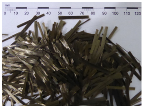
Fig. 1 Chopped basalt micro-fibre used
