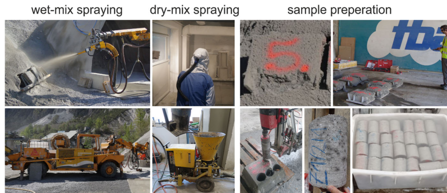
Fig. 1 Impressions of the sample production: from the spraying process (wet and dry) to the aftertreatment and drill core extraction
