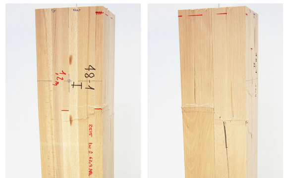
Fig. 4 Failure pattern in a stocky column of strength class GL 48h after reaching a compressive strength of f_{c,0} = 62.9 MPa. Initial failure occurred locally at finger joints
