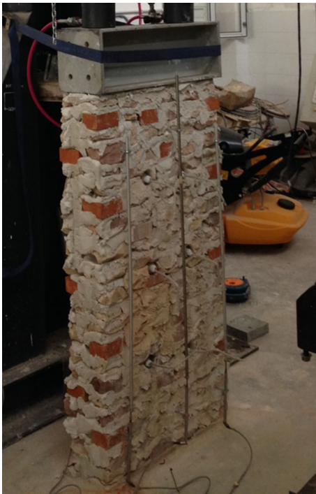
Fig. 8 Compression tests on reinforced panel 4Rf
