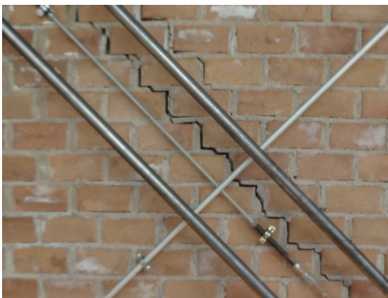
Fig. 5 Detail of failure (unreinforced panel)
