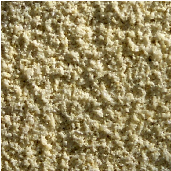
Fig. 6 Surface of sandstone not suitable for the tape test (10 mm × 10 mm in area)
