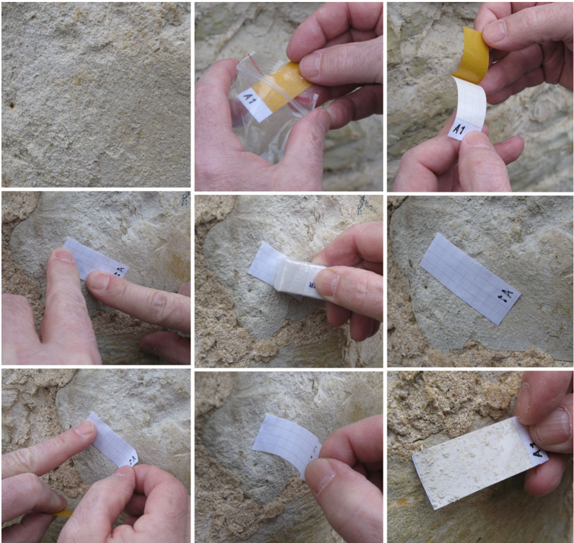
Fig. 14 Peeling test application on an opuka wall-individual steps. The peeled strip is then again covered with the protective layer, inserted back in the plastic bag for transport into laboratory and weighing
