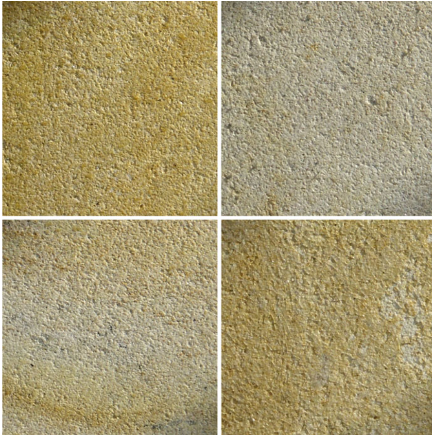
Fig. 5 Surface of opuka stone beam specimens after treatment with lime water ( upper images ), ethyl silicate ( lower left ) and potassium silicate ( lower right ). The individual images cover an area of 10 mm × 10 mm
