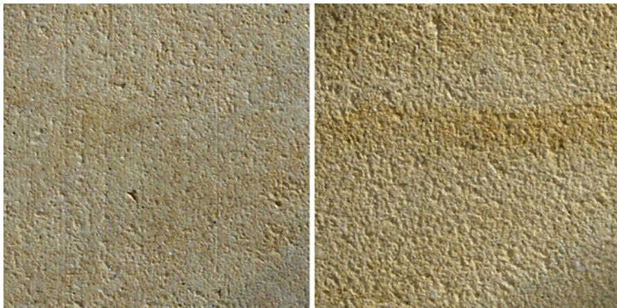
Fig. 4 Surface of opuka natural stone—cube specimen ( left ) and beam specimen ( right ). The individual images cover an area of 10 mm × 10 mm
