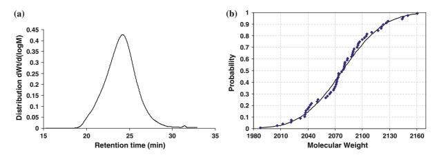
Fig. 8 a Molecular weight distribution plot of an induction-heated bitumen at 110°C. b P–P plot of all the GPC samples, heated at four different temperatures, the original bitumen and the non heated samples
