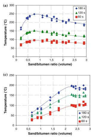
Fig. 6 Maximum reachable temperatures at three different heating times for mastic with different conductive additives content and different sand/bitumen ratios. **a** Conductive additives content 8.76% (steel wool). **b** Conductive additives
