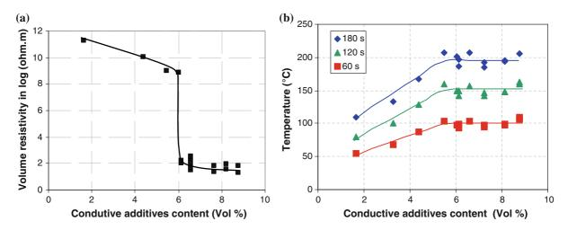
Fig. 7 a Volume resistivity versus conductive particles content for mastic with sand-bitumen ratio 2.25. b Maximum reachable temperatures at three different heating times for different volumes of fibers
