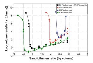
**Fig. 5** Effect of sand-bitumen ratio on the electrical resistivity of the system for different conductive particles-bitumen ratios [1]
