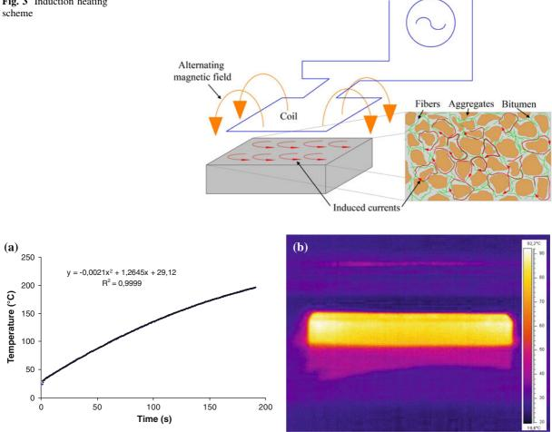
Fig. 4 a Heating curve for a sample with 5.66% steel wool (related to the volume of bitumen) and sand-bitumen 1.60. b Infrared Image of one sample during the induction heating
