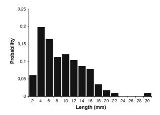
Fig. 1 Chopped steel wool lengths distribution
