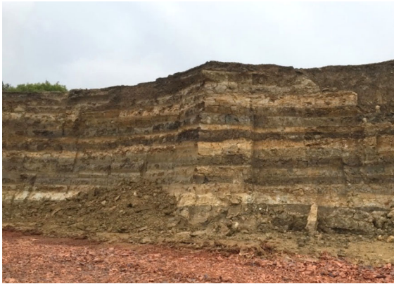
Fig. 1 Photograph of a stockpile with layers of different types of clays, which can then be extracted by digging vertical slices from the stockpile to homogenise the clays
