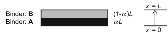
Fig. 2 Conceptual description of geometry and coordinate system for diffusion analysis >L thickness, x distance, \infty relative amount of A
