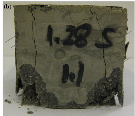
Fig. 9 The fracture modes of mortars: (a) without steel fibers and (b) with steel fibers
