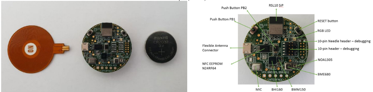
Figure 1. Sensors included in the RSL 10 platform and their measurement range (top). Bottom left: RSL10 platform: NFC antenna (left), platform (middle), battery supply (right). Bottom right: RSL10 platform with main components.
