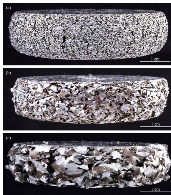
Figure 7: Permeability-tested open-cell Al foams after compression tests for pore (a), (b), and (c).
