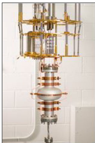
Dilution refrigerator set with an aluminum cavity for device testing at Fermi National Accelerator Laboratory. Credit: Ryan Postel.
