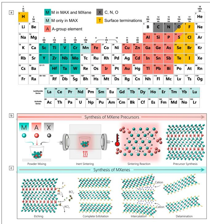
**Figure 1.** The compositional space and synthesis of MAX and MXene phases. (a) The periodic table of elements with marked elements that can be the M, A, X, and T in MAX phases and MXenes. (b) A schematic showing the high-temperature reactive sintering of the MAX phase. (c) A schematic of selective etching of the A-group elements in a MAX crystalline structure to form an exfoliated MXene and intercalation with cations to delaminate MXene particles into single 2D sheets.<sup>10</sup>
