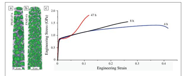
**Figure 7.** Dual functionality of an FeNiAlTi MEA. (a) Coarse- and (b) fine-distributed precipitates serve to strengthen the material while simultaneously modulating the transition of fcc-austenite to bcc-martensite. (c) After annealing heat treatments at 700°C between 4 and 47 h, the resulting materials exhibit yield strengths of ~800 MPa, tensile strengths up to ~1.8 GPa, and ductilities of more than ~40% failure strains.<sup>57</sup>
