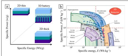
**Figure 1.** Ragone plots of (a) solid-state battery architectures illustrating the enhanced performance of a 3D nanocomposite system over a 2D planar film, (b) state-of-the-art lithium-ion battery technologies.<sup>5</sup>
