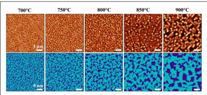
**Figure 5.** Atomic force microscope images (top) and Kinetic Monte Carlo simulations results (bottom) for the LiMn $_2$ O $_4$ -Li $_{0.5}$ La $_{0.5}$ TiO $_3$  nanocomposite growth at a deposition rate of 20 Hz for different growth temperatures. <sup>31</sup>
