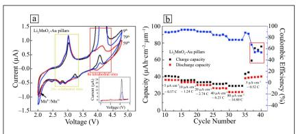
**Figure 3.** (a) Cyclic voltammograms of  $\text{Li}_2\text{MnO}_3$ –Au vertically aligned nanocomposite film with potential 20  $\mu\text{V}$  s<sup>-1</sup> sweep rate at 9th, 59th, and 79th cycle. (b) C-rate performance test at different current densities. <sup>30</sup>
