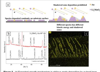
**Figure 2.** (a) Expected growth mechanism in oblique angle deposition by pulsed laser deposition. (b) Out-of-plane x-ray diffraction pattern of  $\text{Li}_2\text{MnO}_3$ –Au vertically aligned nanocomposite film on both  $\text{Al}_2\text{O}_3$  and Au-buffered stainless steel substrates grown at 750°C and 0.067 mbar oxygen pressure. (c) Energy dispersion x-ray mapping for Au confirming the elemental distribution and the pillar formation. <sup>30</sup>
