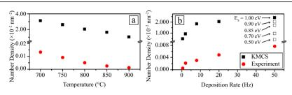
**Figure 6.** Number density comparison between Kinetic Monte Carlo simulations ( $\blacksquare$ ) and experimental results ( $\bullet$ ) as a function of (a) different substrate temperatures for a 20 Hz deposition rate and (b) different deposition rates for a substrate temperature of 800°C. White squares ( $\square$ ) in (b) represent different  $E_S$  values used during simulations.<sup>31</sup>
