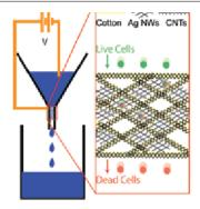
Schematic of the filtration device showing the three components used and the testing technique used for evaluation. NWs is nanowires and CNT is carbon nanotube. Reproduced with permission from Nano Lett. 10 (9) (2010) DOI: 10.1021/nl101944e; p. 3628. © 2010 American Chemical Society.
