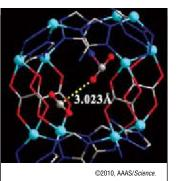
(MOFs) are considered to be some of the best candidates for capturing CO<sub>2</sub>. A study has now revealed crystallographic details of the chemical interaction of carbon dioxide with amine functional groups in MOFs. Computations were in good agreement with experimental results. The results show that an
