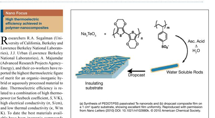
$(\sim 400 \,\mu V/K)$ , but relatively low electrical conductivity and high thermal conductivity. The research team has shown that Te nanorods can be synthesized in situ into a highly electrically conductive, thermally insulating polymer (PEDOT: PSS,  $\sigma > 100$  S/cm,  $\kappa \sim 0.2$ W/m<sup>2</sup>K) in a water solution (see figure).
