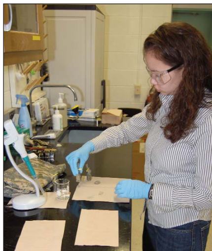
Christina Diaz, a doctoral candidate at Cornell in Juan Hinestroza's group, prepares nylon-cotton camouflage fabric coated with colloidal polystyrene particles through convective and electrostatic self-assembly. Her goal is to make the fabric invisible to someone wearing night vision goggles.
