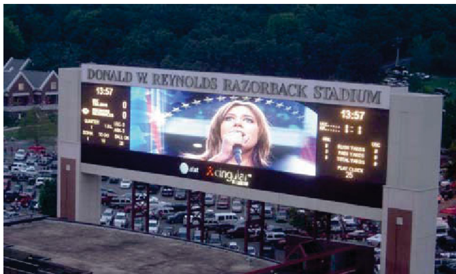
Figure 6. One of the largest LED screens in the world: the Donald W. Reynolds Razorback Stadium replay screen in Arkansas. The screen contains 2.5 million LEDs.
