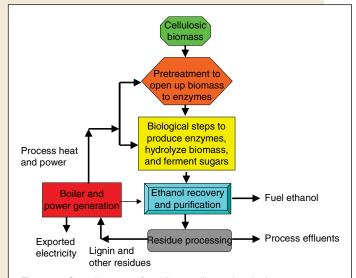
Figure 1. Overall process flow diagram illustrating the important operations in the biological conversion of cellulosic biomass to ethanol.
