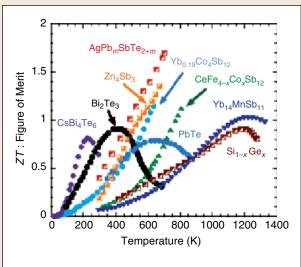
**Figure 1.** Figure of merit (*ZT*) as a function of temperature for several high-efficiency bulk thermoelectric materials.
