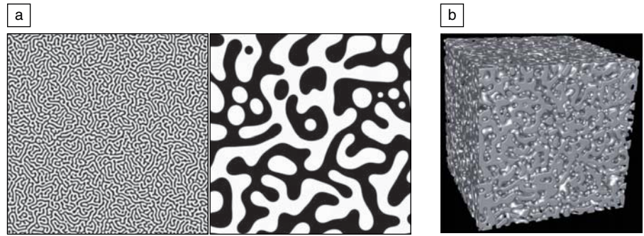
Figure 1. Illustration of differences between two-dimensional (2D) and three-dimensional (3D) simulations of microstructural evolution following spinodal decomposition with half of the material belonging to one phase (white) and half the other (black). (a) An early 2D microstructure is complex and has extensive connectivity over the characteristic length scale of the microstructure (top). However, as coarsening proceeds, the connectivity over the characteristic length scale decreases, and clearly isolated regions (particles enclosed in the other phase) are formed (bottom). (b) In three dimensions, the microstructural evolution following spinodal decomposition proceeds without changes in connectivity over the characteristic length scale of the microstructure. This figure is adapted from Reference 20.
