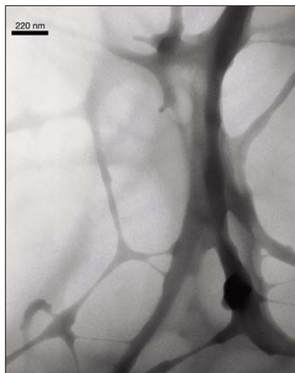
Figure 1. Transmission electron micrograph of a conductive polymer poly(di(oxytrioxadecane)fluorine) single-walled carbon nanotube film. The sample was prepared by microtoming the bulk composite film.
