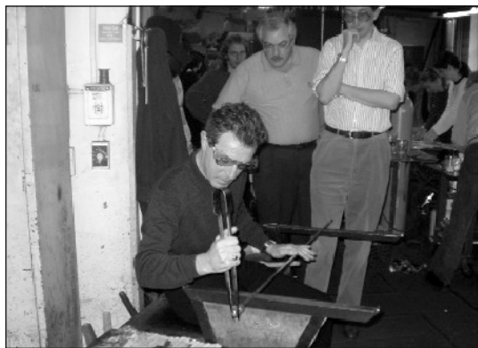
Peter Houk of the MIT Glass Lab begins to build a millefiori cane (or multicolored rod) as observed by Andrew Shortland (Oxford) and others during a workshop held in the Materials Science and Engineering Department at MIT.
