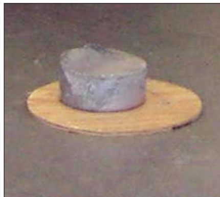
Figure 1. An aluminum ingot (14 cm in diameter; 7.62 cm thick) that has been melted in the microwave furnace.
