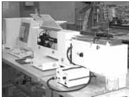
Figure 1. Automated laboratory particle size and shape distribution analyzer.
