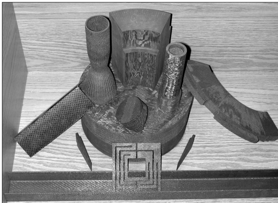
Figure 1. Components fabricated by the in situ rapid densification process include brakes, nozzles, pistons, hypersonic leading edges, heating elements, and structural components.
