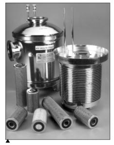
**High-Capacity Vacuum Inlet and Exhaust Trap:** The MV Multi-Trap<sup>®</sup> Model IC from MV Products is designed for collecting solids in LPCVD, MOCVD, WCVD, and metal etch processes. It provides >200 in.<sup>2</sup> (1300 cm<sup>2</sup>) of surface area. Two customizable filtration stages condense and collect heavy particulates. The vacuum inlet and exhaust trap has >500 in.<sup>3</sup> (8000 cm<sup>3</sup>) of space to accumulate solids. Contact: sales@massvac.com; www.massvac.com.
