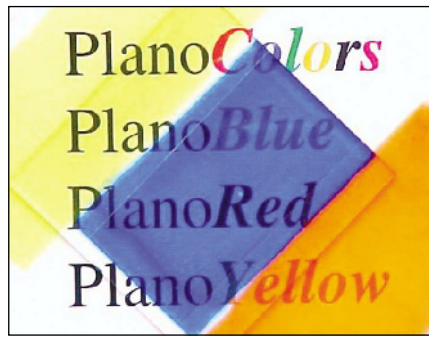
Figure 2: Photograph of transparent, colored nanocomposite Planomer® coatings (showing yellow, blue, and orange) with 5 wt% clay homogeneously dispersed in the solid coating material. The layer thickness is 10–15 \mu\text{m} .
