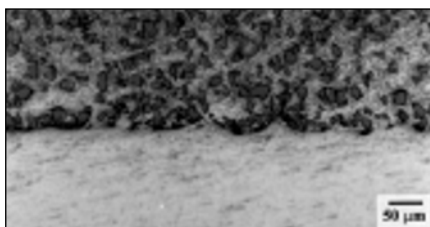
Figure 2: Cross section of a dissimilar joint of Al-6082 alloy and an Al/SiC particulate composite made using the temperature gradient bonding method.
