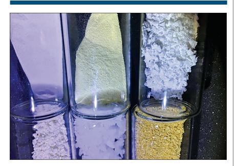
Yttria-stabilized zirconia ceramic oxide serves a critical role in US aerospace and defense industries, as thermal barrier coatings made from this material deliver superior heat resistance and thermal control in jet engines. The Defense Logistics Agency maintains a strategic stock-pile of the rare-earth element yttrium. Credit: Nicholas Burlingame/Defense Logistics Agency.
