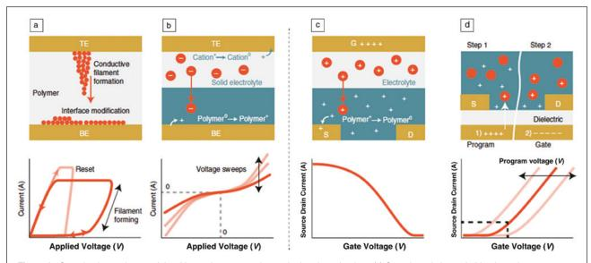
**Figure 2.** Organic electronic materials with conductance tuning and related mechanism. (a) Organic resistive switching based on conducting filaments or interface movements. (b) Redox-based switching with a counter redox reaction in a two-terminal configuration. (c) Redox-based switching in organic electrochemical transistors. (d) Conductance tuning based on nanoparticle charge-trapping.<sup>47</sup>
