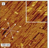
Atomic force microscope images showing the self-assembly of proteins on mica surfaces in presence of 3M KCI: highly packed 2D alignment of short protein rods (a), long nanowires (b), and hexagonal lattices (c). The inserts are zoom-in images and the fast Fourier transform of the hexagonal lattice, respectively. Credit: Nature.
