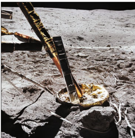
Left: Panel array leaning on the footpad of the lunar module on Apollo 16, which included General Electric experiments to capture cosmic ray tracks in Lexan and phosphate glass. Credit: NASA. Right: Robert L. Fleischer in his office at Union College. Items in the background include images of particle tracks, particle detector “book ends,” and a mannequin with glasses representing the study of eye glasses. Credit: Elizabeth L. Fleischer.
