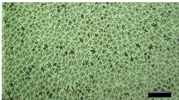
Figure 1. Lithium metasilicate crystals embedded in a Li-depleted \text{CaO-Li}_2\text{O-SiO}_2 glass matrix. Scale bar = 100\ \mu\text{m} . 2
