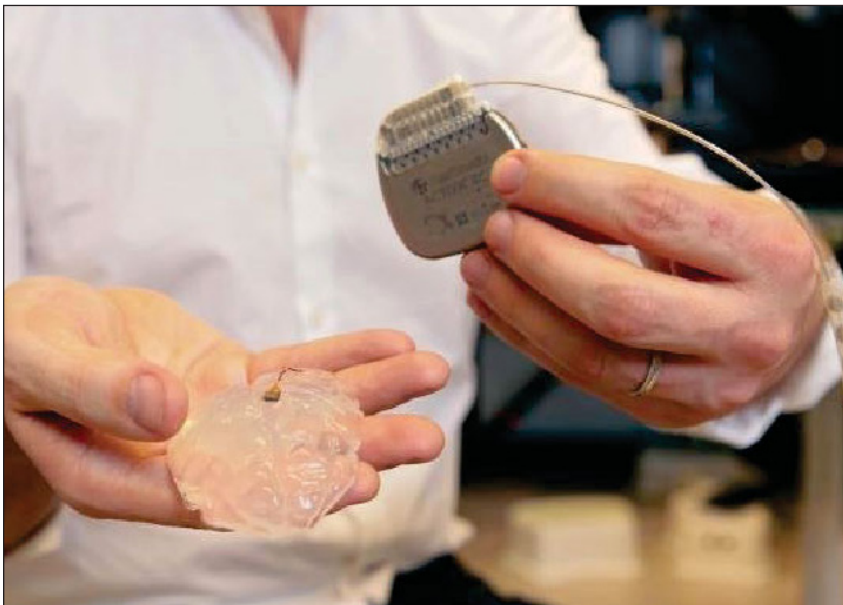
The brain-spine interface works by first decoding signals from the motor cortex into intentions and then using electrical pulses to target specific circuits of the spinal cord that ultimately drive locomotion. Shown here: a pulse generator and a silicon model of a primate’s brain with an attached microelectrode array. Credit: Alain Herzog, EPFL.
