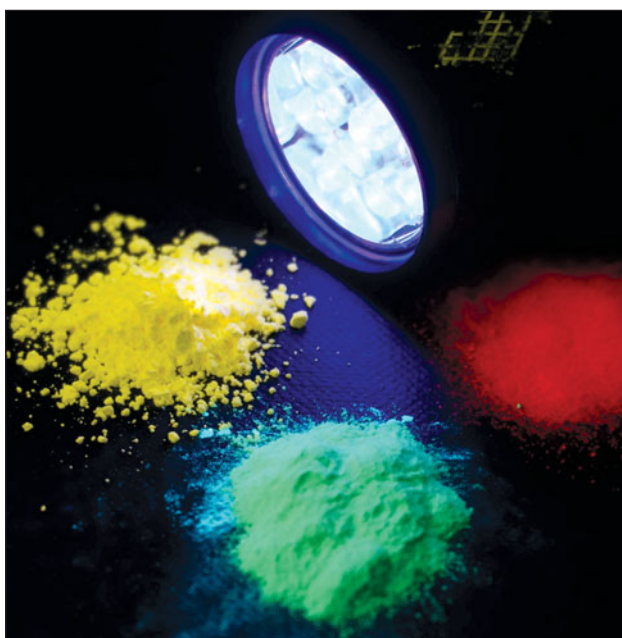
Red, yellow, and green luminescent phosphors and a blue (In,Ga)N LED emitting at 450 nm. Credit: Andries Meijerink, University of Utrecht.
